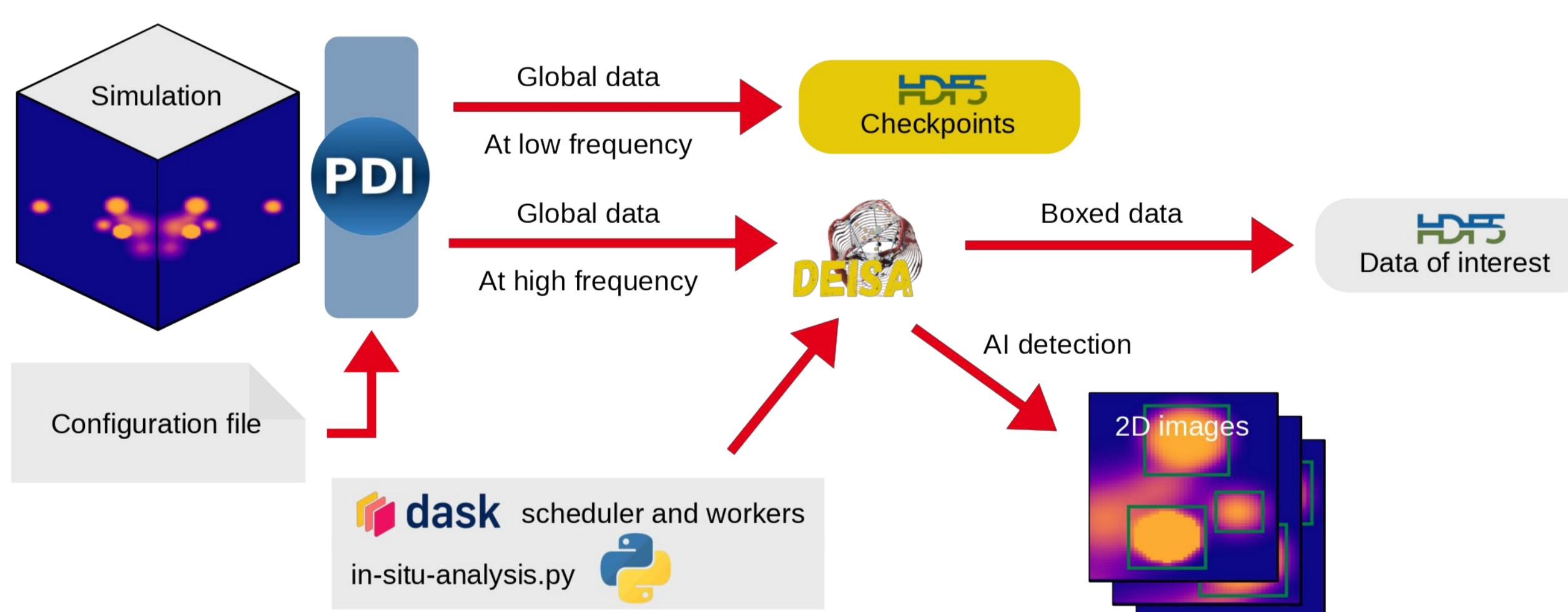
Example of advanced data analysis using PDI and DEISA in an AI workflow.
