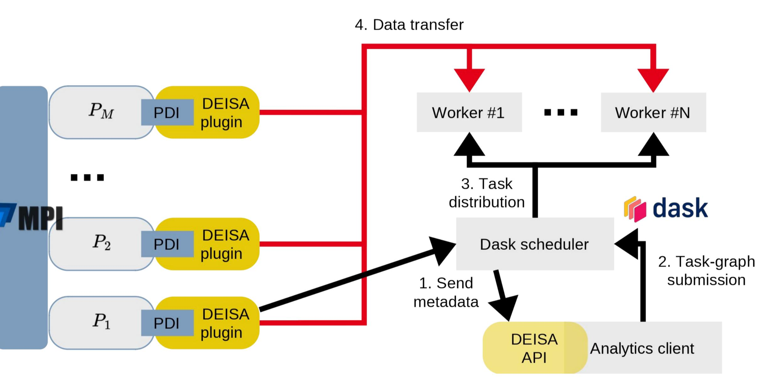
Coupling an MPI application with M processes to a Dask instance running N workers [3].
