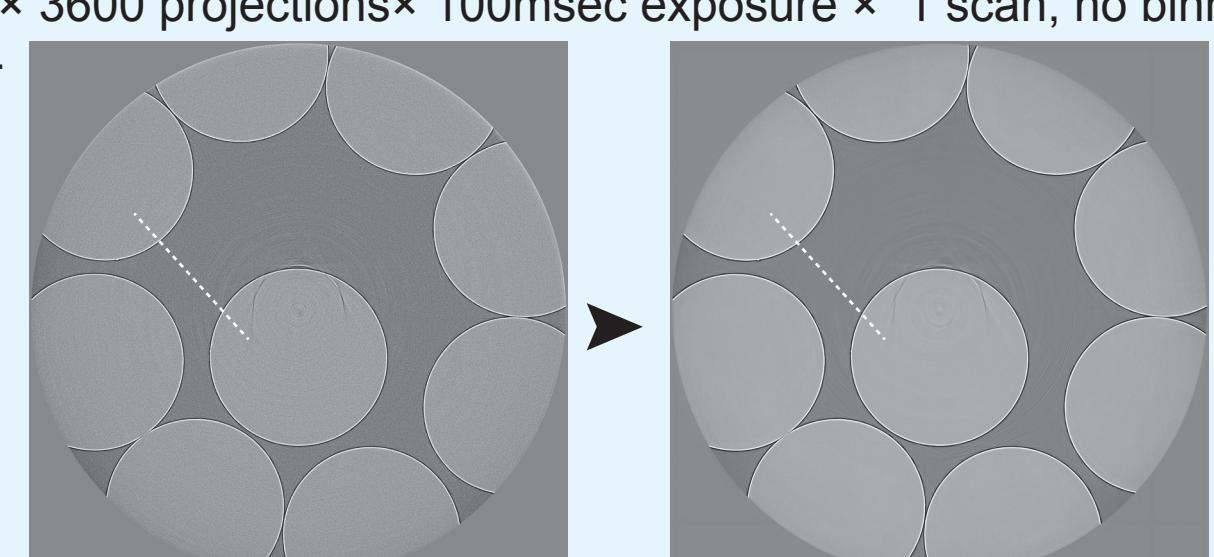
Sample: a star sand (foraminifera), Measured at BL28B2, Energy: 50 keV (by multilayer monochromator). Acquired with 4K-resolution camera (ORCA-Fire), with FOV 4432x2368 pixels, x 3600 projections x 200msec exposure x 1 scan, no binning. Pixel size: 90 nm/px.
