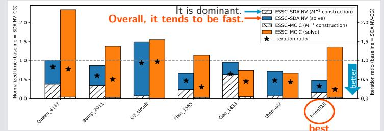
**Note:** The total computation time consists of the time required for building the preconditioner on a CPU and the time required for solving  $k_t$  systems on a GPU.
